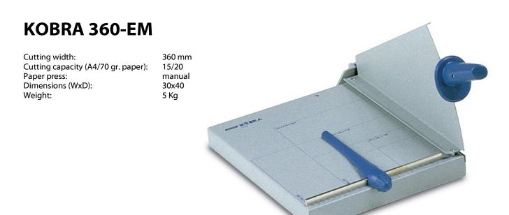
High performances desk-top guillotine with manual paper press. Equipped with the innovative "**SUPER CUT**" system featuring special carbon hardened steel blades and counter-blades unaffected by the wearing action of the materials to cut, for long-lasting cutting operations with the same cutting precision through the years.
